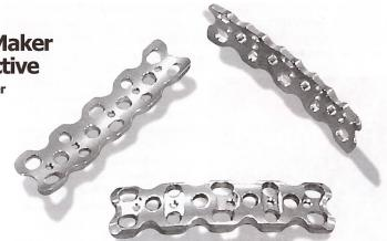
■ Like many implants, these spinal plates have no straight lines. The geometry of such medical components often reflects the natural curves and irregular shapes of the human body. They are manufactured by Criterion Tool & Die in Brookpark, Ohio, and were programmed with PartMaker
